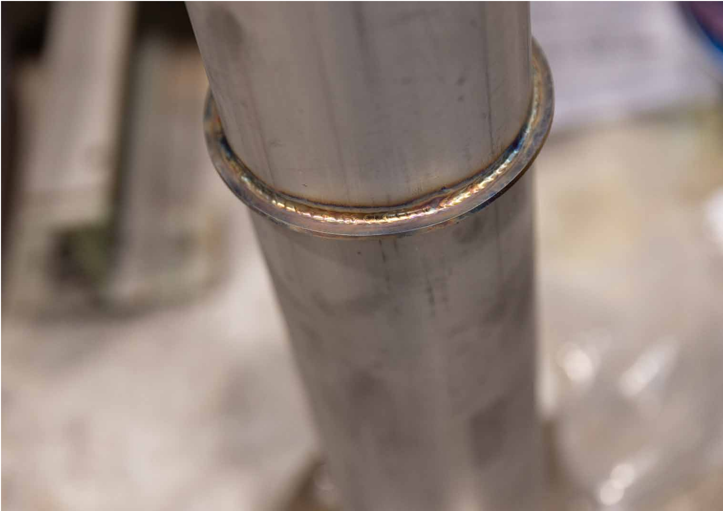
Fillet welding in a rotating device for pipe construction
